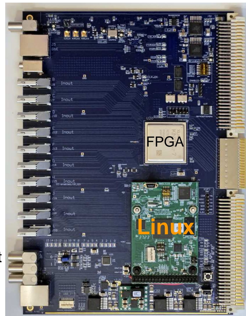
Logic & Trigger Module Serving 320 Channels
