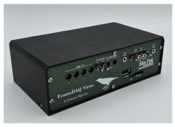
The FemtoDAQ Vireo is a compact, low cost, dual-channel data acquisition system. It uses a embedded Single Board Computer running Linux for data recording and instrument control. It provides two digitizer channels, an FPGA, logic I/O's for connecting to external devices, and a detector bias supply for use with silicon photomultipliers, PIN diodes, and similar detectors.
