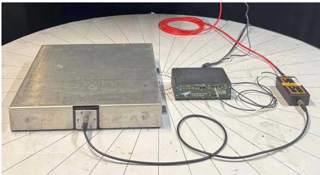
Figure 2. The 15"x15"x2" plastic scintillator + PMT in a metal box (middle) powered via HV splitter box (far right) is delivering negative pulses to the Vireo digitizer. The triggering and signal processing was performed online in real time by Vireo, forming a complete and modern Nuclear Physics experimental system. No external electronics was used other than the photomultiplier HV supply.
